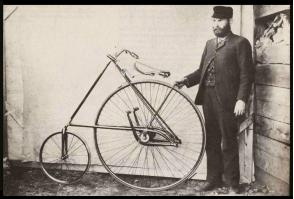
wheel for steering. The Star was driven by ratchet drive, had a hand brake and a sprung leather seat.
